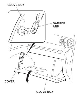
18. Open the glove box. Remove the two stops by releasing the two retaining tabs for each stop. Remove the glove box (two screws).
