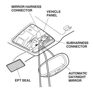
25. Route the terminal from the mirror harness under the headliner toward the right side of the vehicle.
