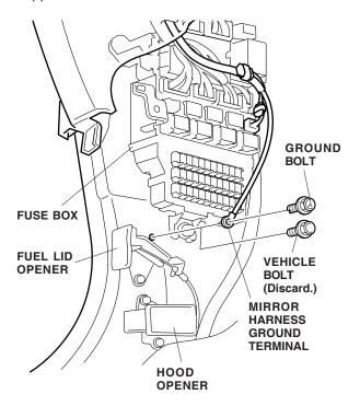
34. Secure the mirror harness to the vehicle harness using two wire ties.
