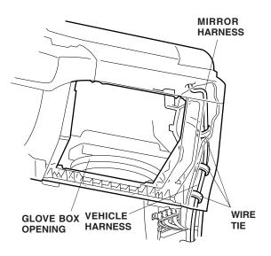
29. Using isopropyl alcohol on a shop towel, clean the right front "A" pillar area where the mirror harness will attach. Attach the mirror harness to the right front pillar using four cushion tapes.
