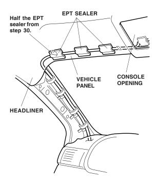
38. Install the wire cover from the mirror to the headliner.
