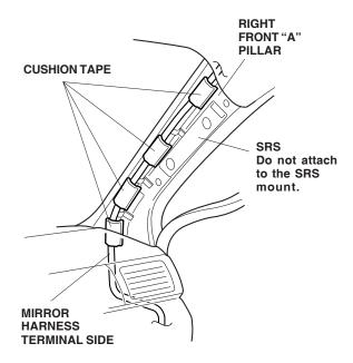
30. Using isopropyl alcohol on a shop towel, clean the headliner area where the mirror harness will attach. Using scissors, cut two EPT sealers in half. Using three halves of EPT sealers, attach the mirror harness to the vehicle panel.
