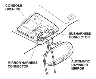
24. Attach the subharness/mirror harness connector to the vehicle panel with one EPT sealer. Position it as far forward as possible.
