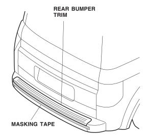
Using isopropyl alcohol on a shop towel, clean the rear bumper where the trim will attach.
