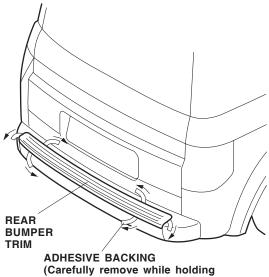
ADHESIVE BACKING (Carefully remove while holding pressure on the trim. After attaching, hold the trim firmly against the rear bumper with the palm of your hand.)
