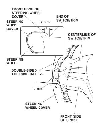
5. Align the rear edge of the steering wheel cover to the back of the steering wheel spoke as shown. Attach the steering wheel cover to the steering wheel with the double-sided adhesive tape.
