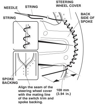
8. After lacing the string through the holes in the steering wheel cover at the back side of the spoke, pull the string tight so the cover wrinkles slightly at the edge. Best fitment results are obtained by lacing up the steering wheel cover tightly.
