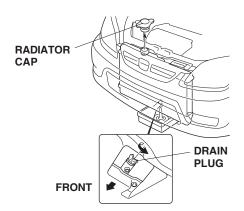
Remove the radiator cover (one bolt and seven clips).
