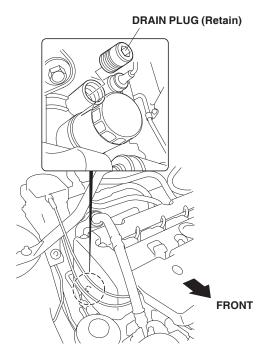
5. Install the engine block heater with the aluminum washer into the bolt hole using a 24 mm socket Torque the engine block heater to 60 N·m (44 lb-ft).
