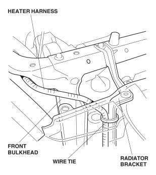
10. Secure the heater harness to the radiator bracket with the one wire tie.
