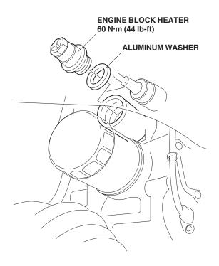
Plug the connector of the heater harness into the engine block heater, and route the heater harness over the engine. Secure the heater harness to the vehicle harness with one wire tie in the area shown.
