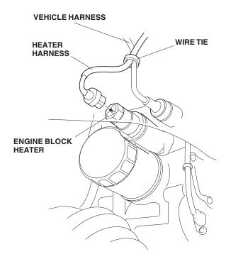
7. Route the heater harness alongside the vehicle harness, and secure the heater harness to the vehicle harness with the three wire ties.
