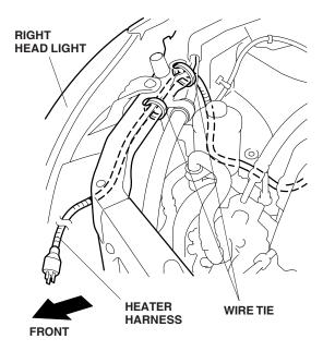
9. Continue routing the heater harness alongside the radiator bracket to the front bumper grille.
