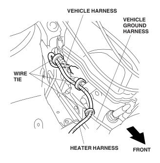
8. Continue routing the heater harness toward the right headlight, and secure the heater harness to the holes of the panels with the two wire ties.
