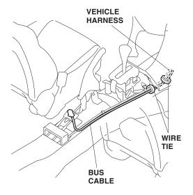
27. Position the center console onto the console bracket, and install the two screws by moving the CD changer right and left.
