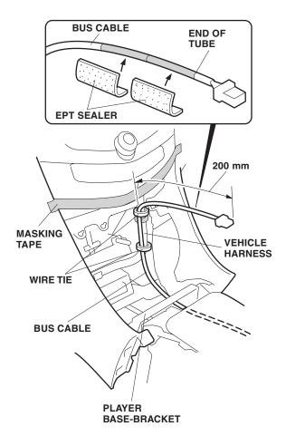
• Plug the BUS cable 14-pin connector into the player.
