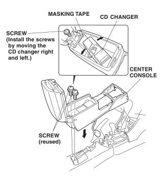
28. Reinstall the center console box inner cover with the BUS cable routed through the cutout.
