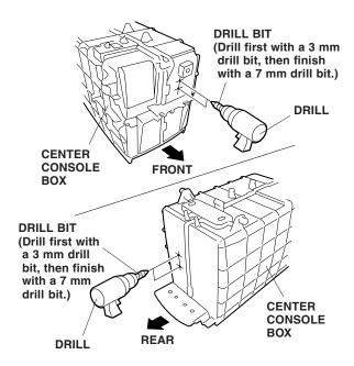
22. Attach masking tape to the center console box in the area shown. Route the CD changer BUS cable out through the lid opening, then carefully slide the CD changer into the console box.
