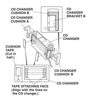
18. Using scissors, cut the cushion tape in half.
