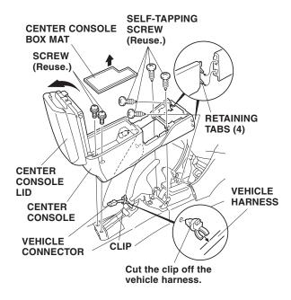
10. Remove the center console rear cover (two self-tapping screws and two clips).
