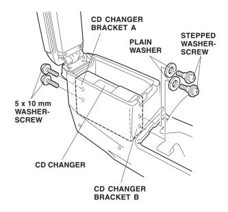
31. Secure CD changer bracket B to the center console with two stepped washer-screws and two plain washers.
