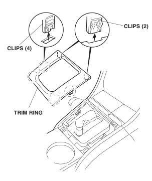
4. Pry up on the beverage holder to release the six clips, and remove the beverage holder.
