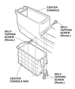
13. Remove the center console box inner cover (one self-tapping screw and release one retaining tab, and two hooks).
