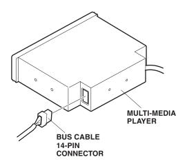
Plug the BUS cable connector into the vehicle connector, and reinstall the player and pocket.
