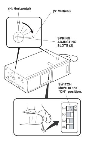
15. If the vehicle is equipped with an in-dash 6-disc CD Changer, use a pin to move the number 2 switch to the "ON" position.
