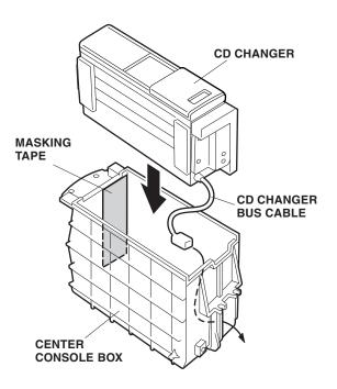
23. Reinstall the center console box into the center console using the four self-tapping screws removed in step 12.
