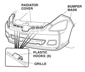
14. Attach the six elastic straps to the inside top edge of the grille opening, and attach the three plastic hooks to the bottom inside edge of the grille opening.
