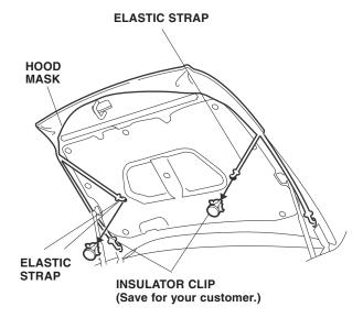
3. Fit the corners of the hood section around the hood, and adjust the mask so it fits smoothly over the edges. Attach the four elastic straps to the holes in the hood.
