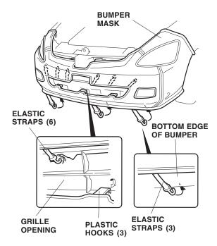
15. Attach the three remaining elastic straps to the bottom edge of the bumper.
