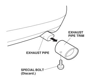
Partially thread the supplied special bolt into the new exhaust pipe trim.
