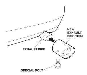
3. With the special bolt on the bottom, slide the exhaust pipe trim onto the exhaust pipe until it bottoms.
